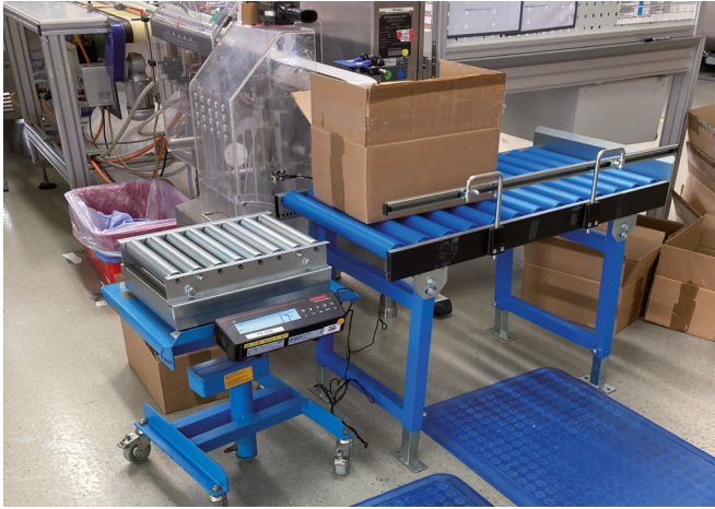
A new roller conveyor and roller scale were installed on one of our lines, eliminating the need for heavy lifting of boxes
